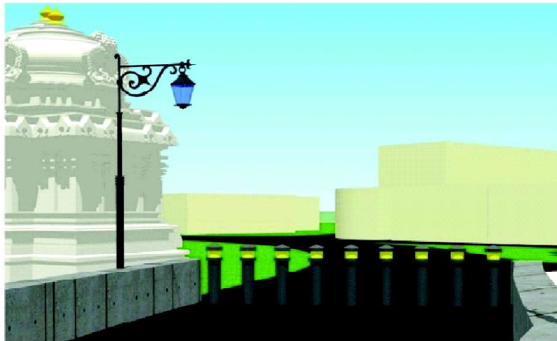
Figure 22: Automatic lowering Bollards
